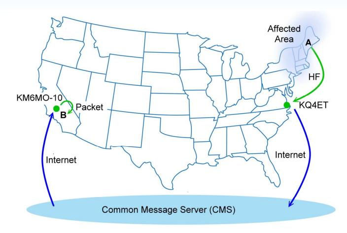
The process is the same as that shown in Example 1. Station A is in an area without standard communications services. It connects by HF to a RMS outside the affected area. Station B connects to a local RMS via packet and the message is retrieved.
